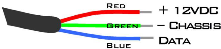
If the tube is to be connected to an ICELED controller supplying both power and data, then the colour coded wires simply connect to the corresponding terminals labelled R, G and B on the chosen output.
