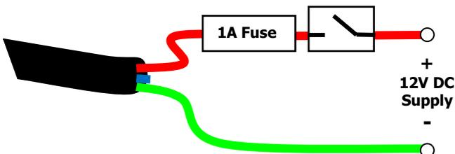
In this case the blue (data) wire is unused and should therefore be insulated or cut off close to the cable end.
